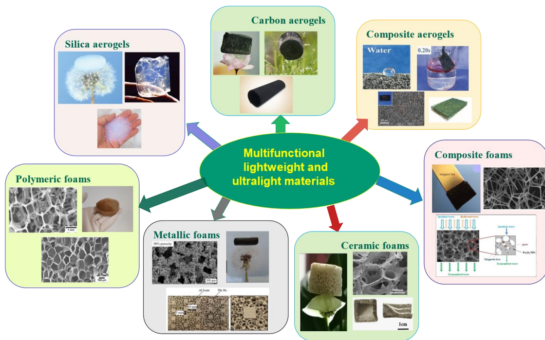
Figure 1. Different types of lightweight and ultralight materials.
